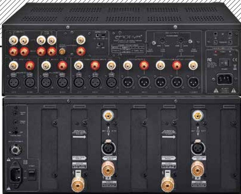
**ABOVE:** The preamp [top] offers six line inputs (four on RCA, two balanced on XLR), one MM/MC phono input, a processor/tape loop, L/R/Sub HT inputs and outputs, plus main outs (RCA and XLR). The power amp [below] has single-ended (RCA) and balanced (XLR) inputs with fully floating (ungrounded) speaker outputs
